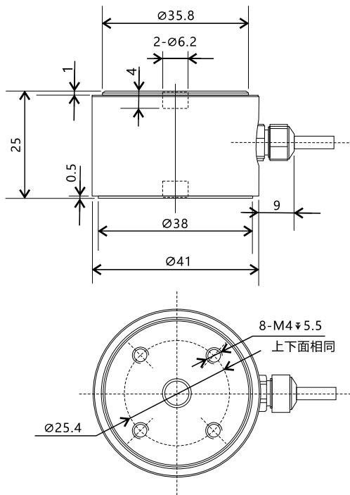
拉压双向 Tension and Compression Load
